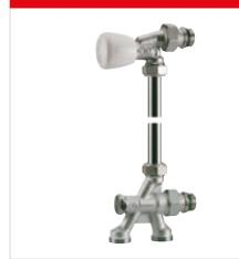
Angled valve and lockshield valve group with thermostatic option and connections from the floor, brass chrome plated, with connection for copper, plastic or multilayer pipe adaptors. For twin-pipe systems. Equipped with adjustable lockshield valve. To be completed with R194 chrome plated connection pipe, Ø16 mm. Connection to the system pipes with R178, R178C, R179 or R179AM adaptors.
