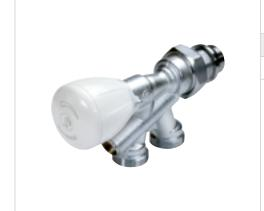
Micrometric valve with thermostatic option, brass chrome plated, with connection for copper, plastic or multilayer pipe adaptors. For single-pipe systems. Equipped with adjustable lockshield valve. Supplied with R171P plastic probe, Ø 12 mm, lenght 450 mm.
