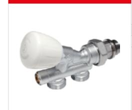
Compact micrometric valve with thermostatic option, brass chrome plated, with connection for copper, plastic or multilayer pipe adaptors. For single-pipe systems. Equipped with adjustable lockshield valve. Supplied with R171P plastic probe, Ø 12 mm, lenght 450 mm.
