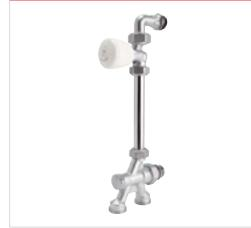
Straight valve and lockshield valve group with thermostatic option and connections from the floor, brass chrome plated, with connection for copper, plastic or multilayer pipe adaptors. For single-pipe systems. Equipped with adjustable lockshield valve. To be completed with R194 chrome plated connection pipe, Ø16 mm. Connection to the system pipes with R178, R178C, R179 or R179AM adaptors.
