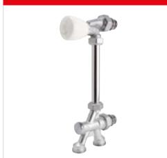
Angled valve and lockshield valve group with thermostatic option and connections from the floor, brass chrome plated, with connection for copper, plastic or multilayer pipe adaptors. For single-pipe systems. Equipped with adjustable lockshield valve. To be completed with R194 chrome plated connection pipe, Ø16 mm. Connection to the system pipes with R178, R178C, R179 or R179AM adaptors.
