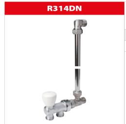
Manual valve and lockshield valve group, brass chrome plated, with connection for copper, plastic or multilayer pipe adaptors. For single-pipe systems. To be completed with R194 chrome plated connection pipe, Ø16 mm. Connection to the system pipes with R178, R178C, R179 or R179AM adaptors.
